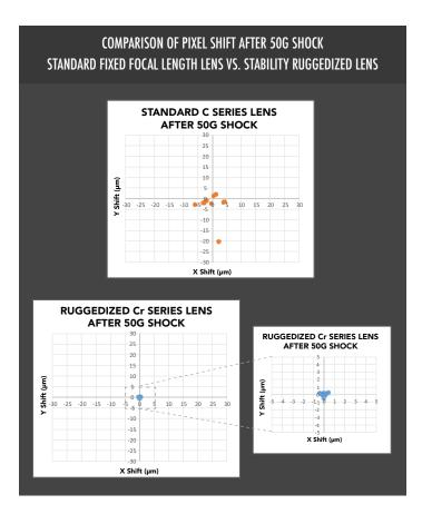
**Figure 3:** While the standard imaging lens (C Series Fixed Focal Length Lens) on the left performs well under normal conditions, 50G of shock causes a pixel shift of more than a single pixel. The Stability Ruggedized Cr Series Lens, on the other hand, experiences less than 1µm of pixel shift after 50G of shock, which is a much smaller shift than the size of a pixel.
